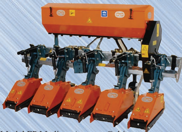
Model FP Medium Acreage Cultivator with Optional Fertilizer Attachment
